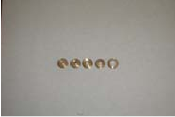
Figure 11. Nozzles of hydro cyclone with different diameters
