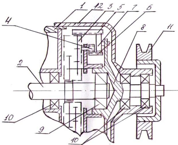
Figure 5. The constructive scheme starting the switching devices
