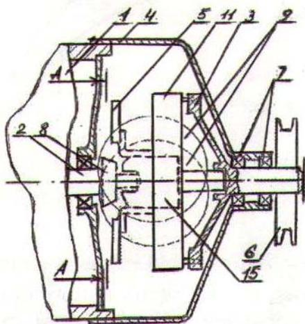
Figure 2. The constructive scheme of actuating unit for starter-generator
