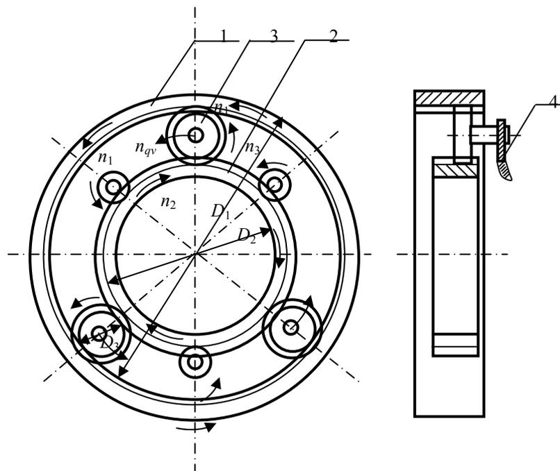
Figure 6. The scheme of placing of external, internal and leading wheels
