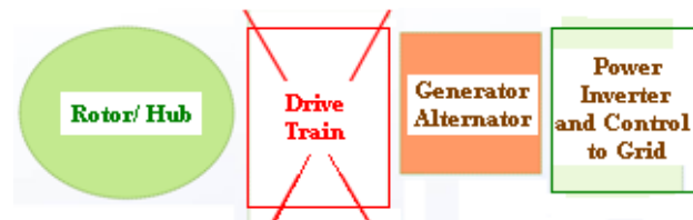
Figure 3. A new trend in turbine configuration
