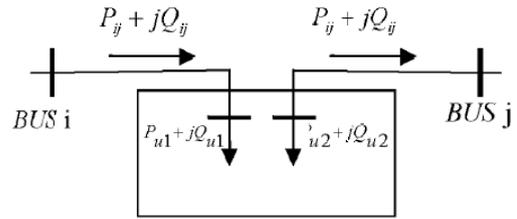
Figure 2. The decoupled model of UPFC
