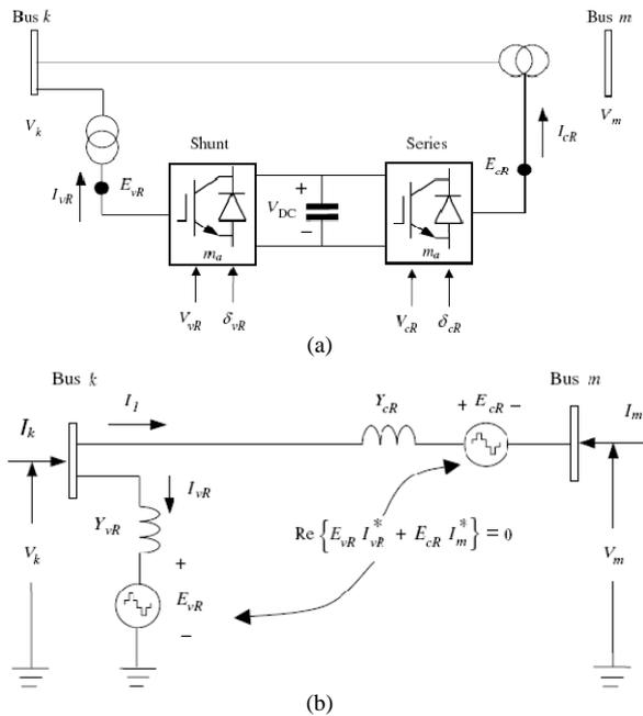
Figure 1. Block diagram of the UPFC system: (a) Two back-to-back voltage source converters (b) Equivalent circuit of a UPFC
