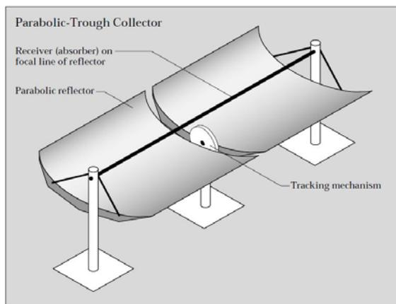
Figure 5. A device that can save and shift sun heat
