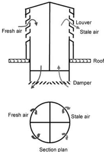
Figure 9. Schematic view of new wind catchers [7].
