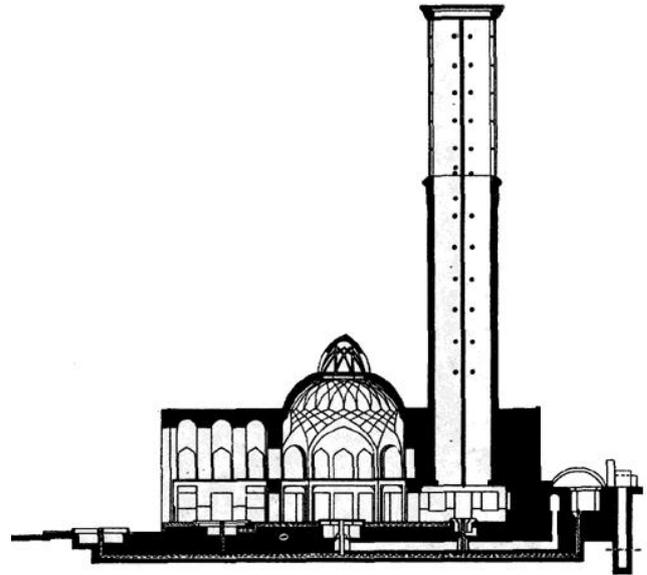
Figure 10. Schematic view of Dolat Abad wind catcher
