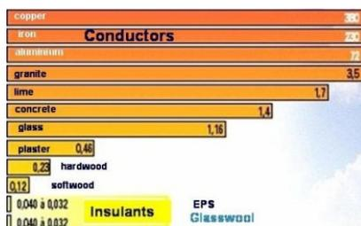
Figure 4. Thermal conductivity levels in different conductors
