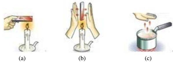
Figure 1. The heat transfer methods: (a) Conduction, (b) Convection, (c) Radiation
