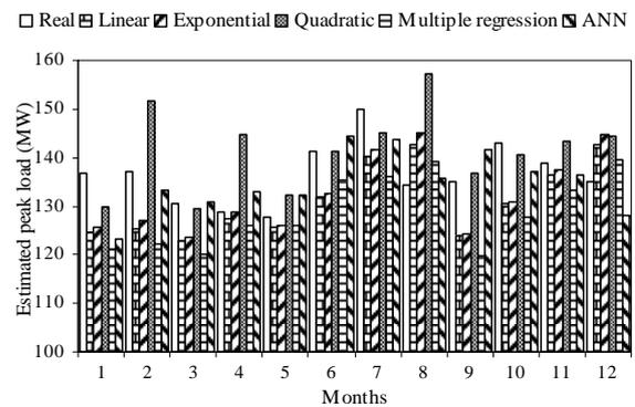
Figure 2. Real and forecasted peak load values for 2008
