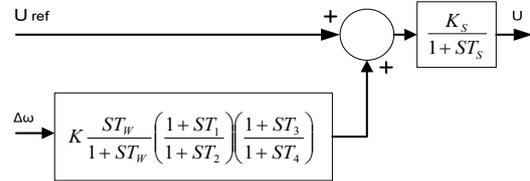
Figure 4. IPFC with lead-lag damping controller
