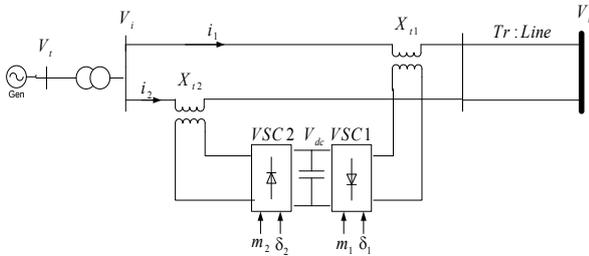
Figure 2. SMIB power system equipped with IPFC
