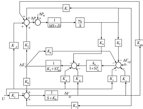
Figure 3. Modified Heffron-Phillips transfer function model for IPFC
