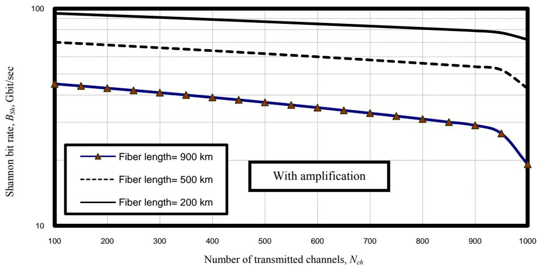
Figure 14. Variations of Shannon bit rate against number of transmitted channels at the assumed set of parameters
