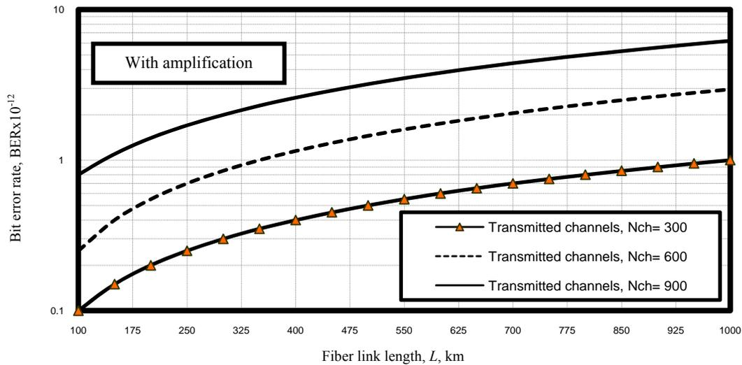
Figure 18. Variations of received bit error rate against fiber link length at the assumed set of parameters
