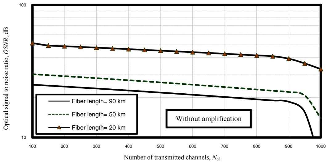
Figure 13. Variations of optical signal to noise ratio against number of transmitted channels at the assumed set of parameters
