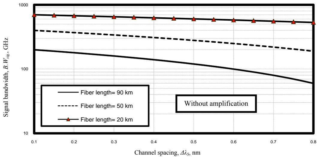
Figure 11. Variations of the signal bandwidth against channel spacing at the assumed set of parameters
