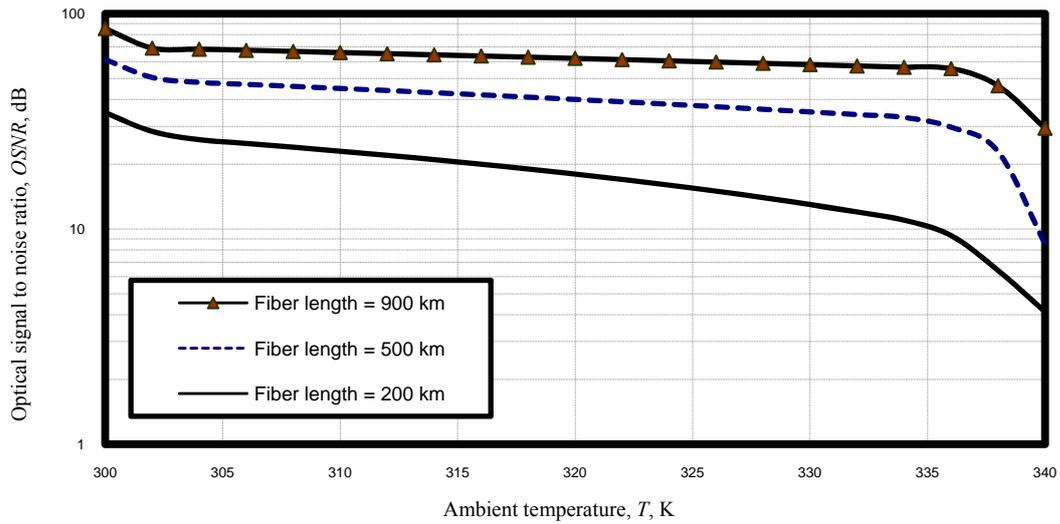
Figure 6. Variations of the optical signal to noise ratio versus ambient temperature at the assumed set of parameters
