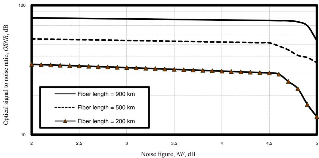
Figure 8. Variations of the optical signal to noise ratio versus noise figure at the assumed set of parameters
