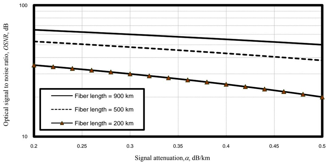
Figure 7. Variations of the optical signal to noise ratio versus signal attenuation at the assumed set of parameters
