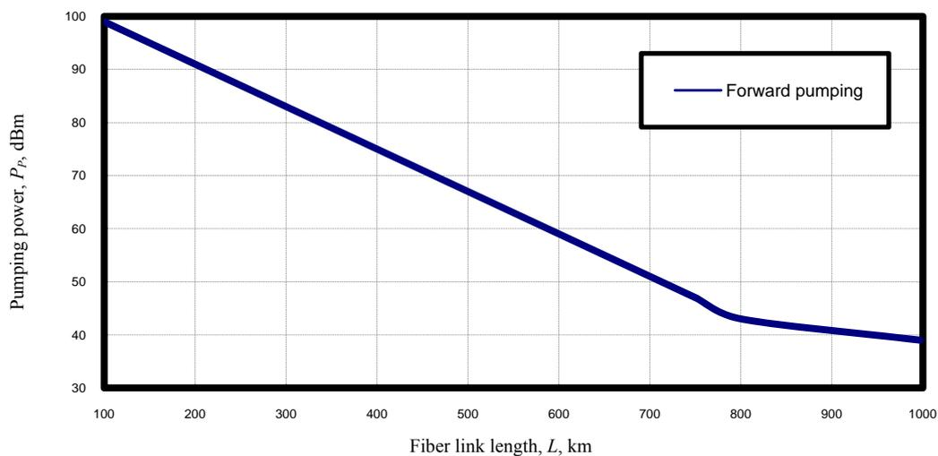
Figure 2. Variations of the pumping power against the fiber link length at the assumed set of parameters
