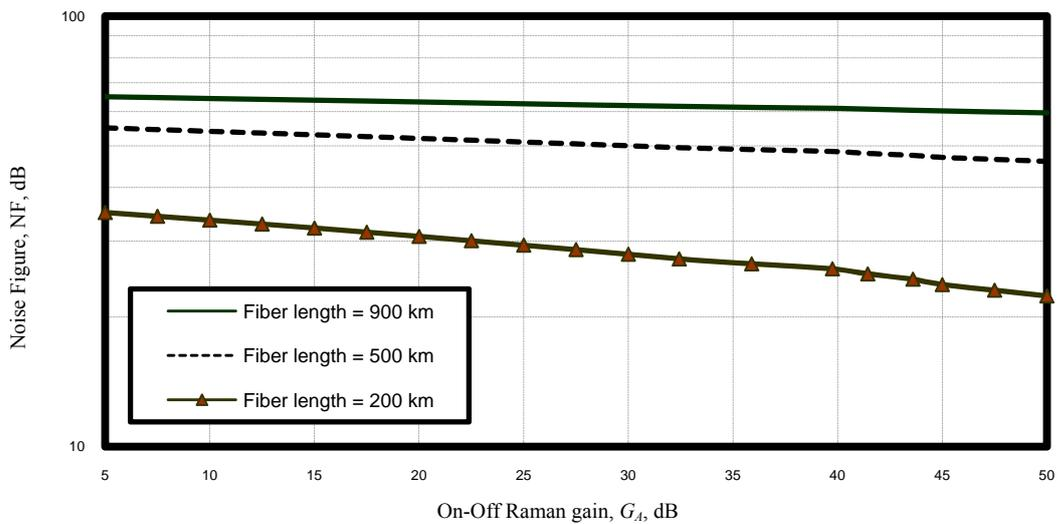
Figure 5. Variations of the noise figure with the on-off Raman gain at the assumed set of parameters
