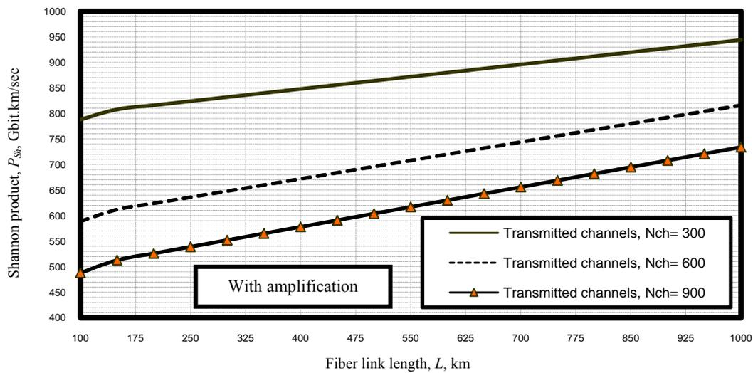
Figure 16. Variations of Shannon bit rate-distance product versus fiber link length at the assumed set of parameters
