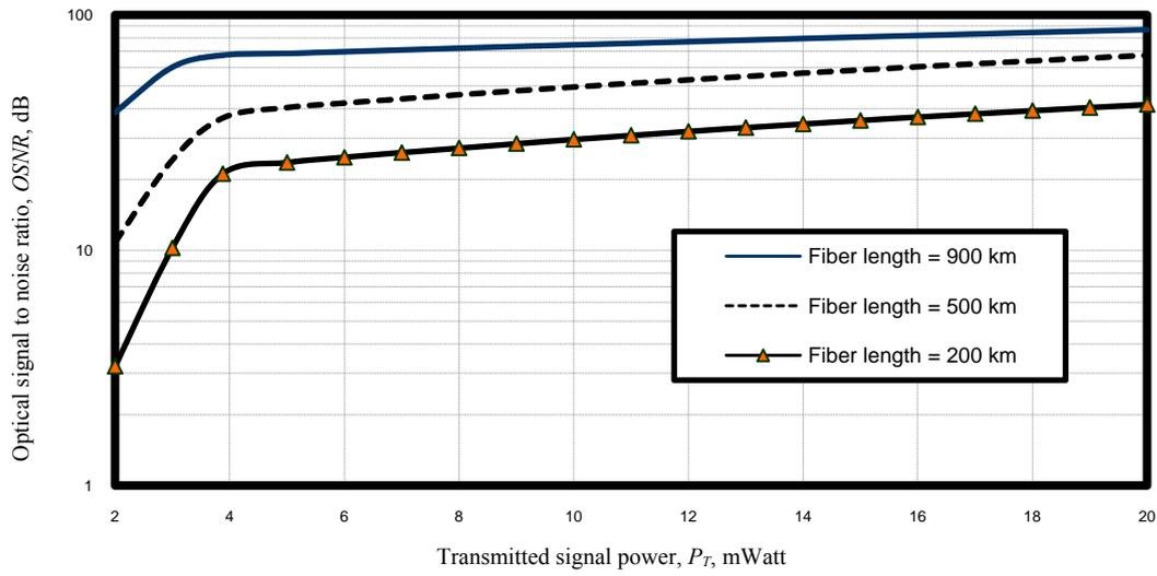
Figure 9. Variations of the optical signal to noise ratio against transmitted signal power at the assumed set of parameters
