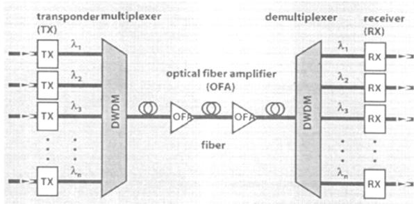
Figure 1. DWDM photonic networks
