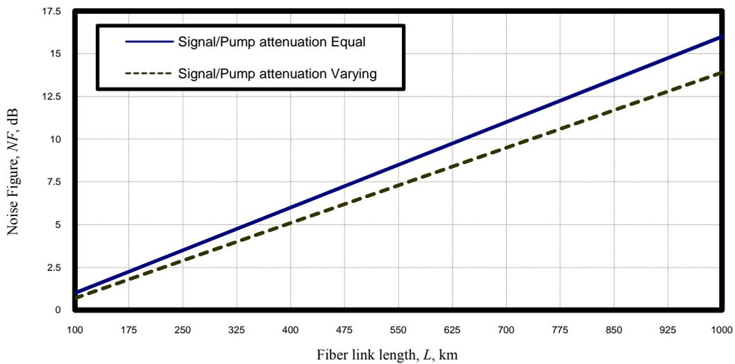
Figure 4. Variations of noise figure against the fiber link length at the assumed set of parameters
