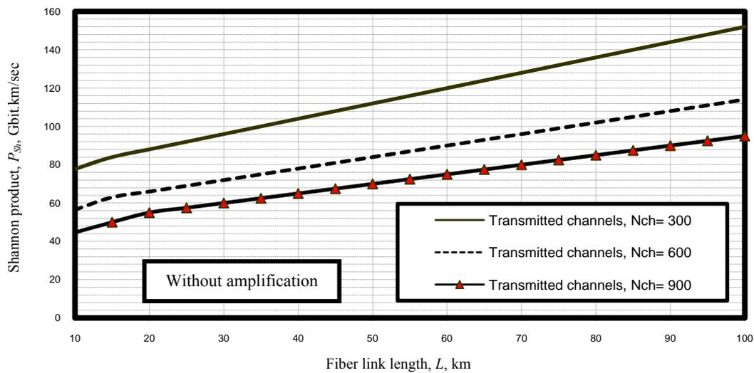
Figure 17. Variations of Shannon bit rate-distance product versus fiber link length at the assumed set of parameters
