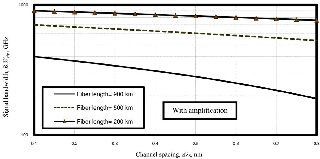
Figure 10. Variations of the signal bandwidth against channel spacing at the assumed set of parameters
