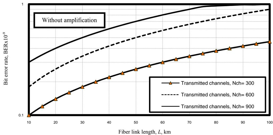
Figure 19. Variations of received bit error rate against fiber link length at the assumed set of parameters
