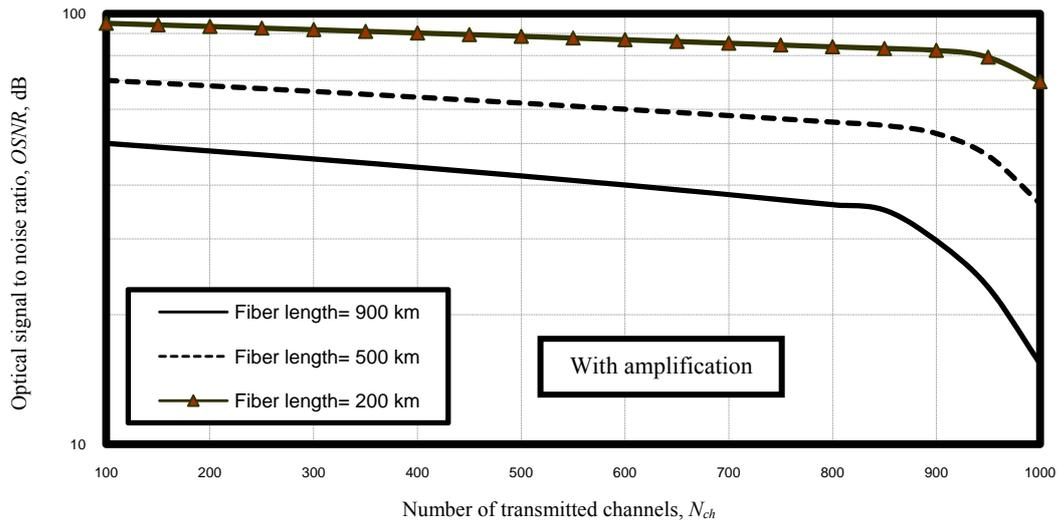
Figure 12. Variations of optical signal to noise ratio against number of transmitted channels at the assumed set of parameters
