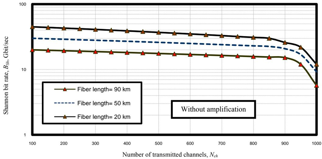
Figure 15. Variations of Shannon bit rate against number of transmitted channels at the assumed set of parameters
