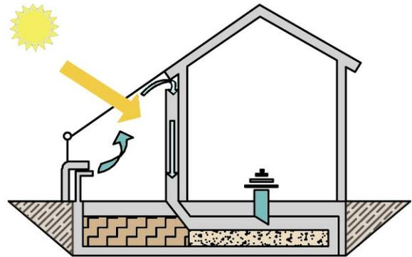
Figure 4. Isolated gain system, storage process
