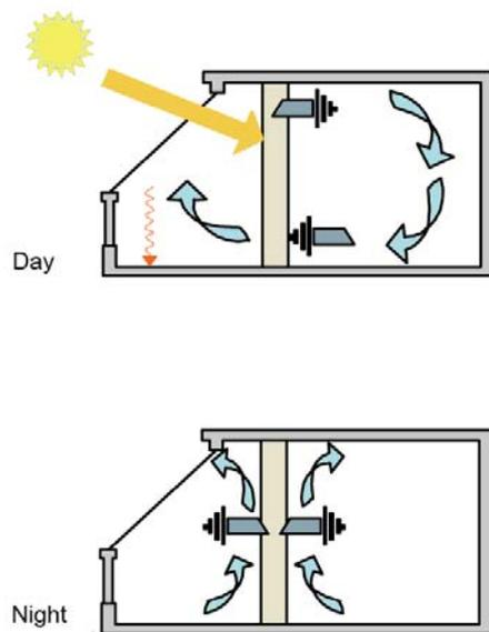
Figure 5. The combination of Trombe Wall of masonry material and greenhouse, the performance in day/night cycle
