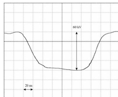
Figure 2. Oscillogram of high voltage pulse
