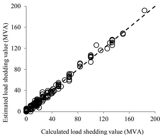
Figure 7. Proposed algorithm accuracy in estimating the load shedding value considering load priority
