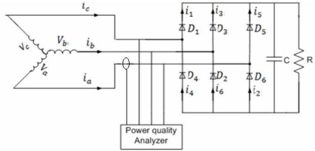
Figure 7. Three phase nonlinear RC load circuit
