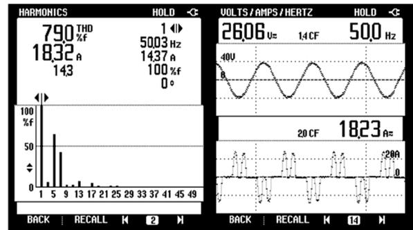
Figure 8. Nonlinear load  $U, I$  waveforms and harmonic spectrum in case 3 [12]
