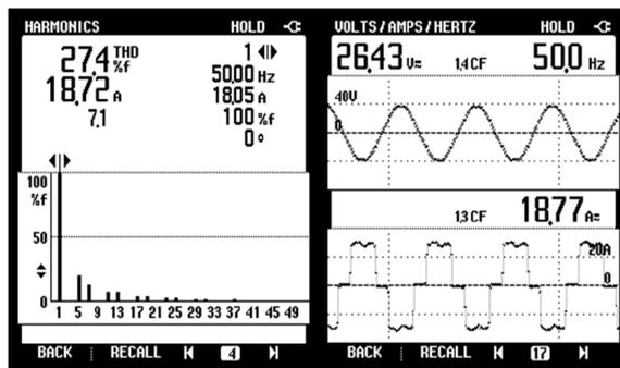
Figure 6. Nonlinear load  $U, I$  waveforms and harmonic spectrum in case 2 [12]
