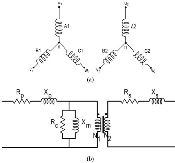
Figure 1. (a) The winding connections (b) per-phase equivalent circuit of a three phase transformer
