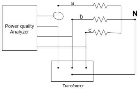
Figure 3. Three phase linear load
