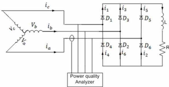
Figure 5. Three phase nonlinear RL load circuit
