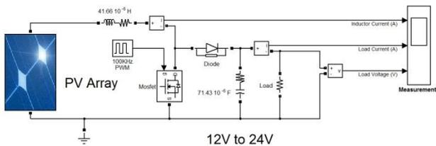
Figure 8. Boost converter, with SimPowerSystems
