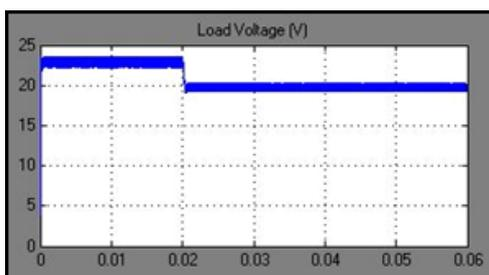
Figure 11. Result simulation boost converter
