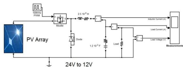
Figure 4. Buck converter, with SimPowerSystems
