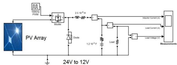
Figure 4. Buck converter, with SimPowerSystems
