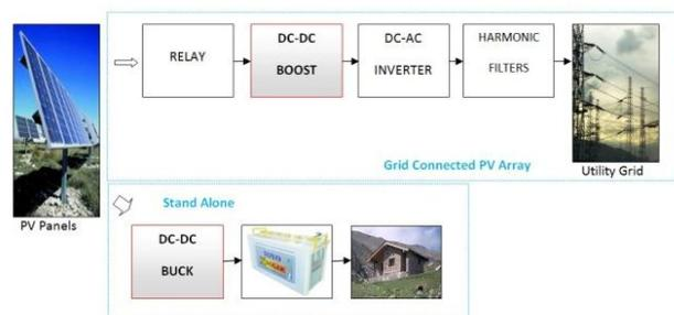
Figure 1. Schematic of the elements of a photovoltaic system
