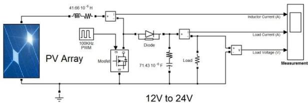
Figure 8. Boost converter, with SimPowerSystems
