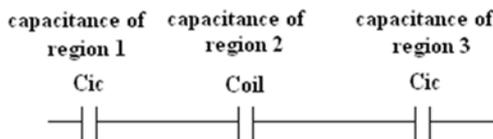
Figure 5. Series combination of capacitances in the distance of two adjacent turns
