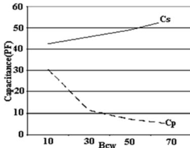
Figure 10. Changes of total series and parallel capacitances due to the changes of  $B_{cw}$
