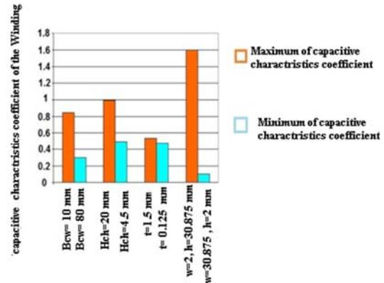
Figure 18. The max and min of the coefficient of  $\alpha$  for the various parameters
