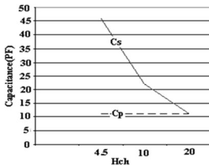
Figure 11. Changes of total series and parallel capacitances due to the changes of  $H_{ch}$
