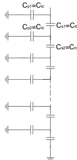
Figure 9. Capacitive network of the layer winding
