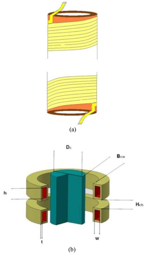
Figure 8. (a) View of a complete layer winding, (b) View of a layer winding with 2 turns
