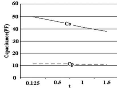
Figure 12. The variations of the total series and parallel capacitances due to the changes of  $t$
