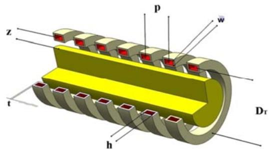
Figure 3. View of a coil with rectangular cross section of turns
