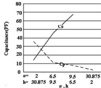
Figure 13. The variations of the total series and parallel capacitances due to different value of  $w, h$
