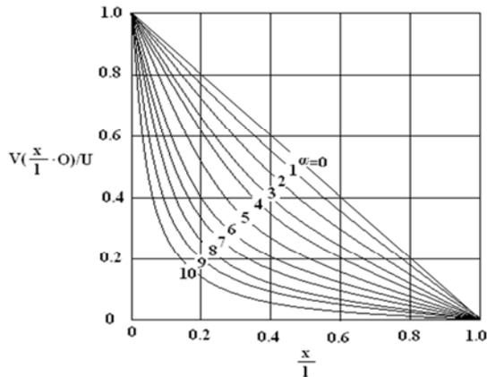
Figure 2. Impact of  $\alpha$  on the initial impulse voltage distribution [2]
