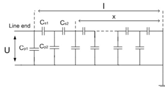
Figure 1. Capacitive network of the transformer winding in time of the strike of the impulse voltage  $U$
