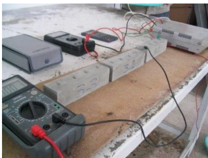
Figure 2. Cement paste bars for resistivity test setup
