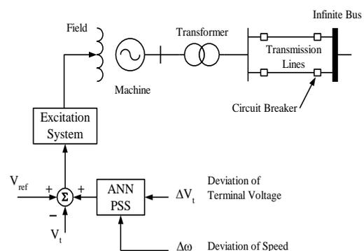
Figure 6. Schematic diagram of 1 machine infinite bus system and MOHBMPSS [4]
