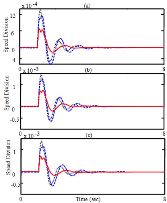
Figure 9. System response by 0.2 pu step increasing the mechanical torque in  $t = 1$ , Solid (Proposed-PSS), Dashed (SPEA-PSS) Dotted (GA-PSS), (a)  $P = 0.8, Q = 0.4, X_e = 0.6$ , (b)  $P = 0.5, Q = 0.1, X_e = 0.6$ , (c)  $P = 1.0, Q = 0.5, X_e = 0.6$
