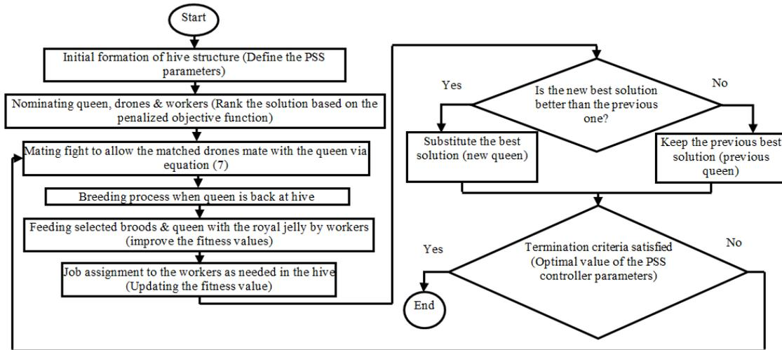
Figure 3. Algorithm and computational flowchart of HBMO [22]
