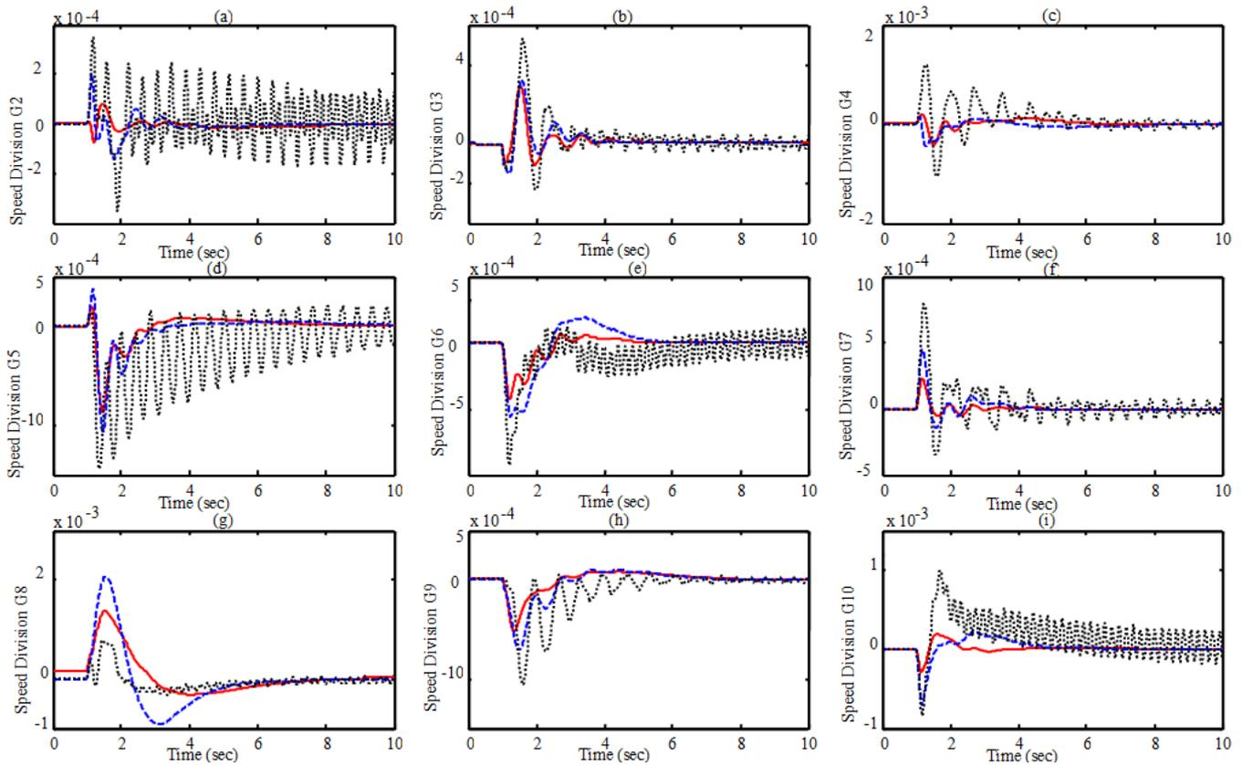
Figure 13. System response under scenario 3 with nominal loading condition, Solid (proposed-PSS), Dashed (PSO-PSS), Doted (C-PSS)
