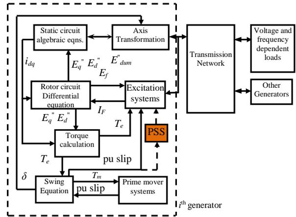
Figure 2. Structure of PSS in power systems [1]
