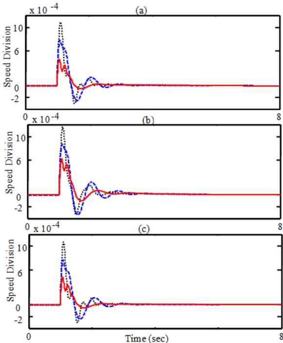
Figure 8. System response by 0.2 pu. step increasing the mechanical torque in  $t = 1$ . Solid (Proposed-PSS), Dashed (SPEA-PSS) Dotted (GA-PSS), (a)  $P = 0.8, Q = 0.4, X_e = 0.3$ , (b)  $P = 0.5, Q = 0.1, X_e = 0.3$ , (c)  $P = 1.0, Q = 0.5, X_e = 0.3$
