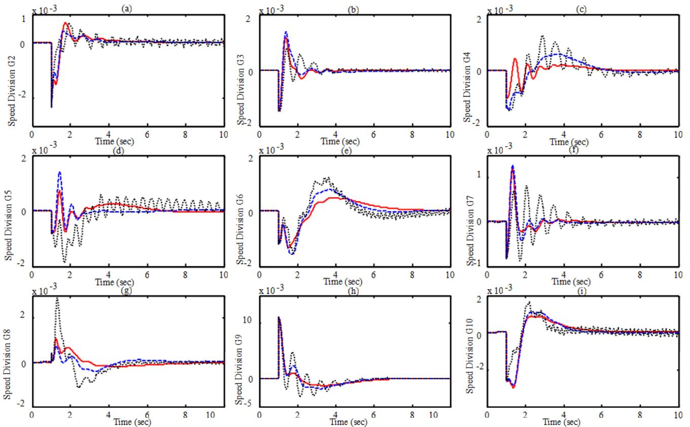
Figure 12. System response under scenario 2 with light loading condition, Solid (proposed-PSS), Dashed (PSO-PSS), Doted (C-PSS)
