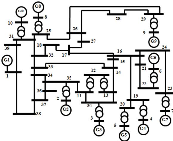
Figure 7. Ten-machine 39-bus new England power system [4]
