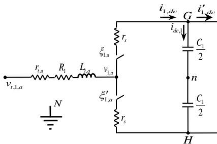
Figure 2. Equivalent circuit of phase a of converter 1
