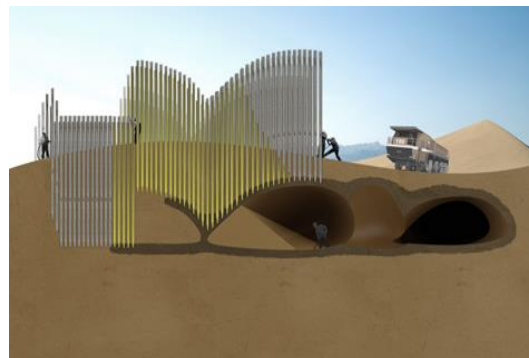
Figure 2. Soil solidification biological method
