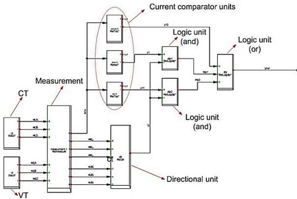
Figure 5. Block diagram of SPCS4D11
