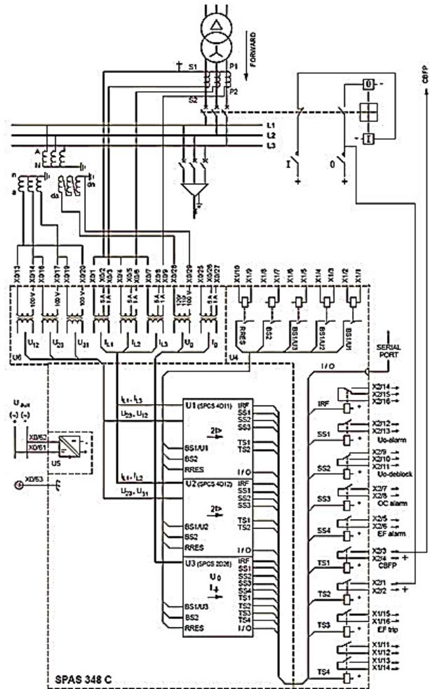
Figure 3. Block diagram of SPAS348C [1]
