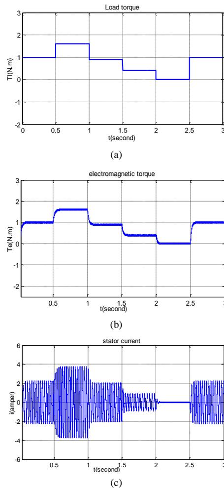
Figure 10. Controller performance in nominal state of PMSM motor in different load for the second Lyapunov function, (a) Load torque, (b) Electromagnetic torque, (c) Stator current of one phase
