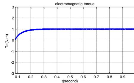
Figure 14. Electromagnetic torque for the proposed controller of the second Lyapunov function under load with deviation parameters in  $L_d = L_q = +30\%$ ,  $J_m = +400\%$
