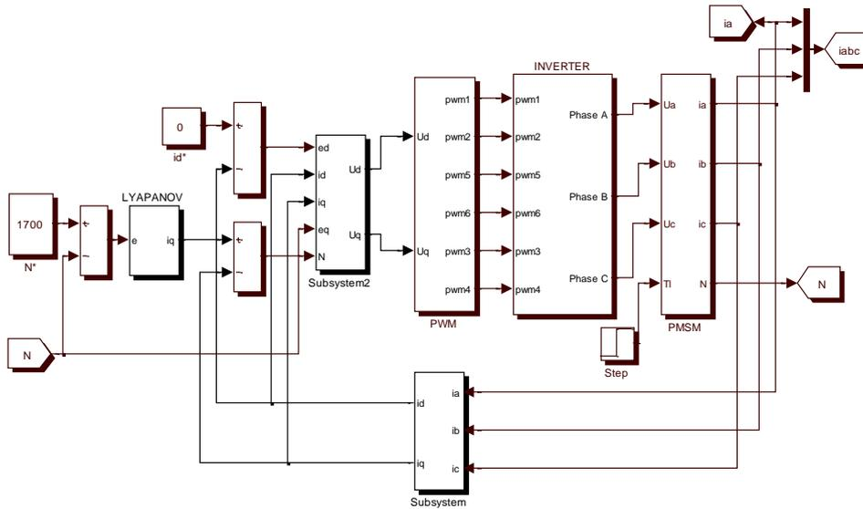
Figure 8. Block diagram of the system for nonlinear control based Lyapunov approach
