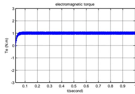
Figure 13. Electromagnetic torque for the proposed controller of the first Lyapunov function under load with deviation parameters in  $L_d = L_q = +30\%$ ,  $J_m = +400\%$
