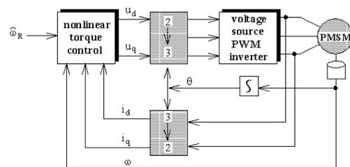
Figure 7. Overall system block diagram related to PMSM motor torque control
