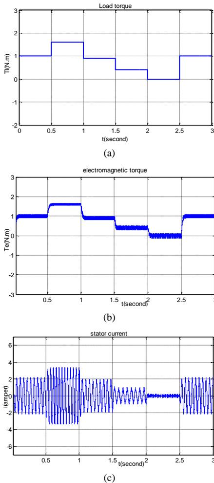
Figure 9. Controller performance in nominal state of PMSM motor in different load for the first Lyapunov function, (a) Load torque, (b) Electromagnetic torque, (c) Stator current of one phase
