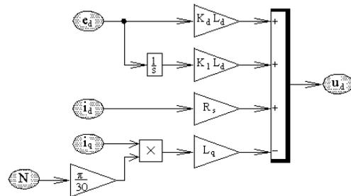
Figure 5. Controller block diagram for  $u_d$
