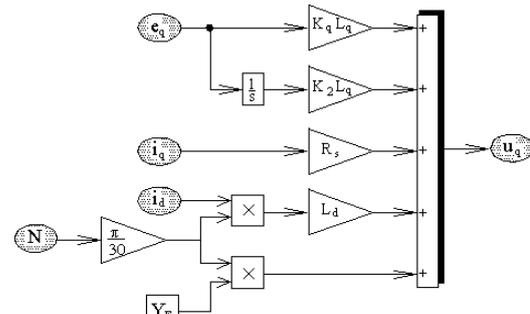
Figure 6. Controller block diagram for  $u_q$
