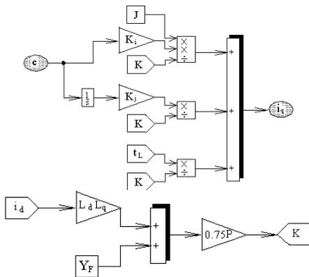
Figure 4. Controller block diagram for  $i_q$
