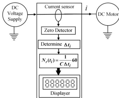
Figure 5. Sensorless speed measurement system
