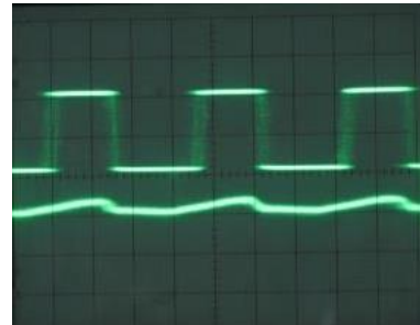
Figure 9. Current waveform of the DC motor in slow speed
