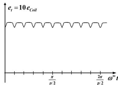
Figure 3. Induced voltage waveform of the DC motor
