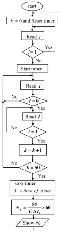
Figure 7. Compute the DC motor speed by microcontroller
