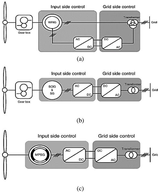
Figure 2. Types of methodology when wind turbine connected to grid
