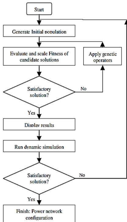
Figure 3. Flowchart of GA for optimal allocate of compensator resources
