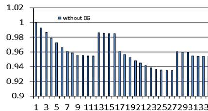
Figure 4. Voltage profile without DG from standard mode of network
