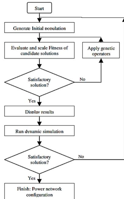
Figure 1. Flowchart of GA for optimal allocate of DG units
