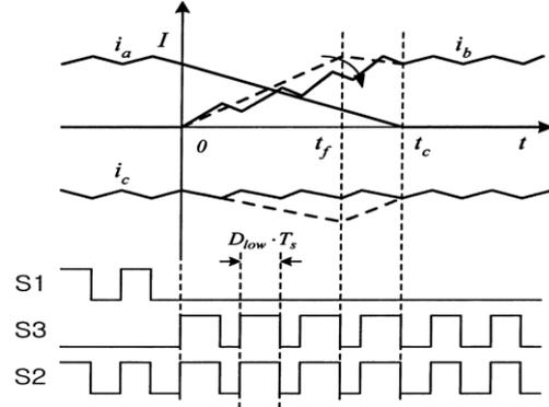
Figure 3. Switching patterns and commutation in low speed [6]
