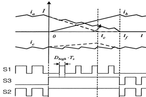
Figure 4. Switching patterns and commutation in high speed [6]
