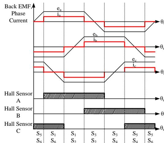
Figure 2. Signal waveforms in the BLDC motor
