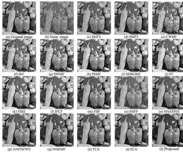
Figure 3. Comparison of the enhanced images for the Peppers by impulse noise density of 50%
