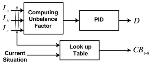
Figure 10. Control block diagram of CV-LLC for unbalance reduction in distribution system
