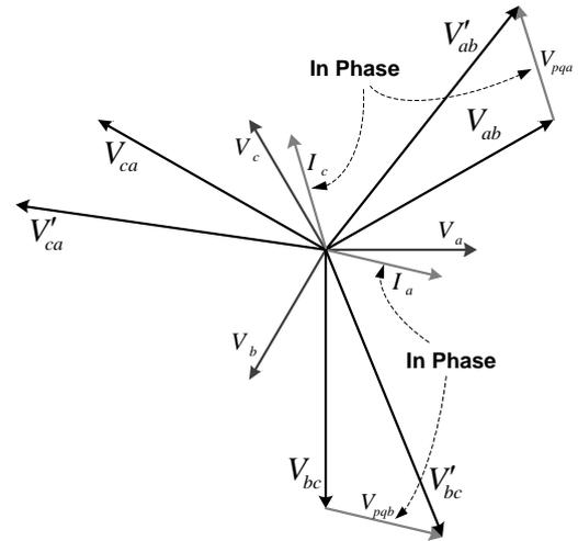
Figure 4. Phasor diagram of V-LLC with current frame control
