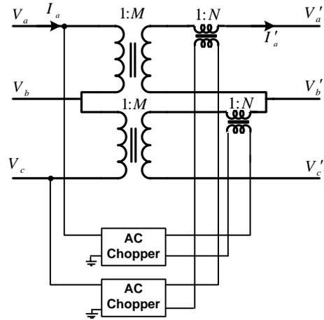
Figure 8. Structure of CV-LLC
