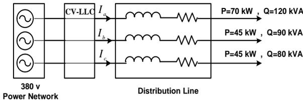
Figure 15. Simulated distribution unbalance network
