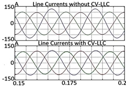
Figure 16. Line currents with unbalance load
