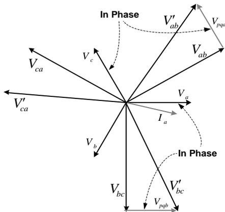
Figure 5. Phasor diagram of V-LLC with voltage frame control
