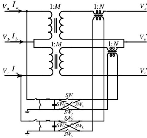
Figure 9. CV-LLC for unbalance reduction
