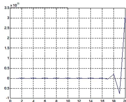
Figure 2. Unstable response of the closed loop system while controlled by a discrete PID controller (excited by a unitary step)
