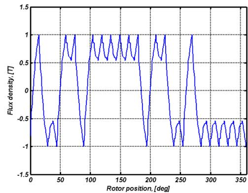
Figure 7. Flux density waveform in one portion of rotor core of 8/6 SRM over a full revolution of rotor
