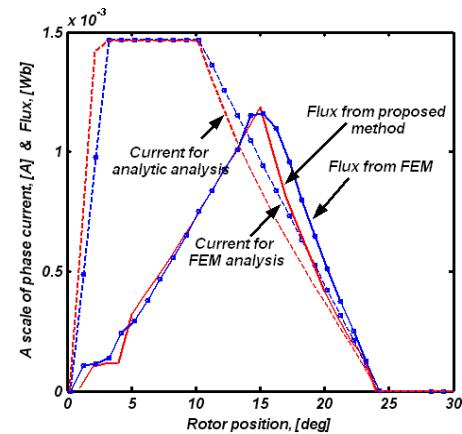
Figure 3. Comparison of stator pole flux and excitation current waveforms of 8/6 SRM for proposed analytical and FE methods
