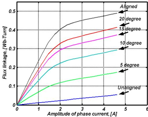
Figure 1. Flux-linkage characteristic of 8/6 SRM at different rotor positions using flux tube method
