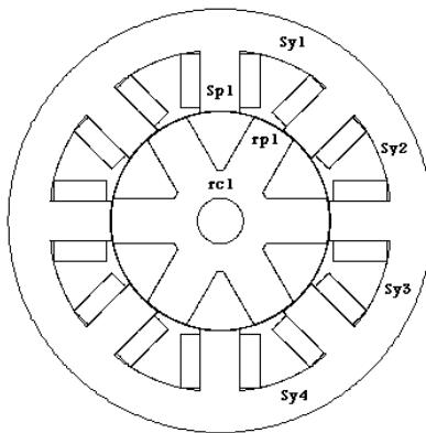
Figure 4. Various sections of 8/6 SRM
