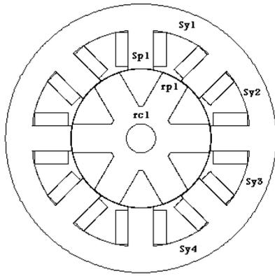
Figure 4. Various sections of 8/6 SRM
