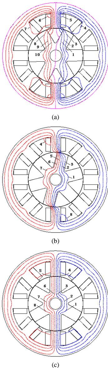
Figure 2. Identification of flux tubes at 8/6 SRM in, (a) region I, (b) region II, and (c) region III
