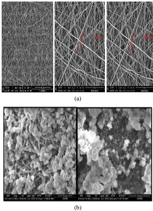
Figure 2. (a) SEM morphologies of the electrospun nanofibers, (b) SEM micrographs of silk-nylon-6 nanofibril array membranes, obtained by the precipitation of calcium-phosphate salts
