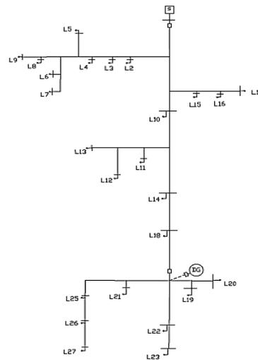
Figure 15. Single-Line diagram of Abidar MV line
