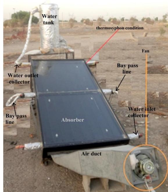
Figure 7. The set-up of dual collector in thermosiphon condition
