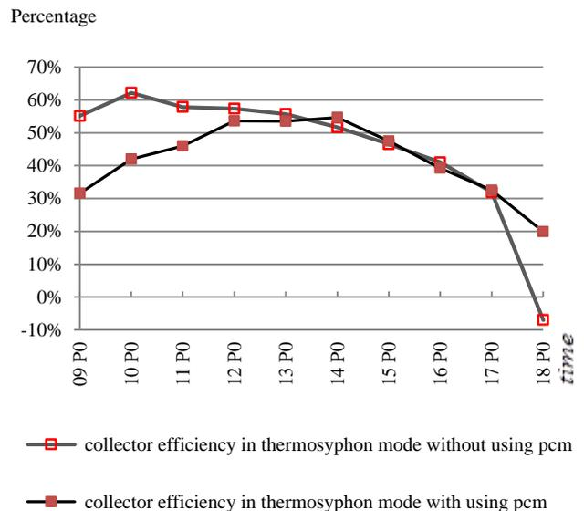
Figure 10. Comparison of the collector efficiency in thermosyphon mode with and without using PCM
