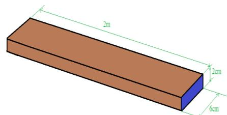
Figure 4. Dimensions of the chamber PCM
