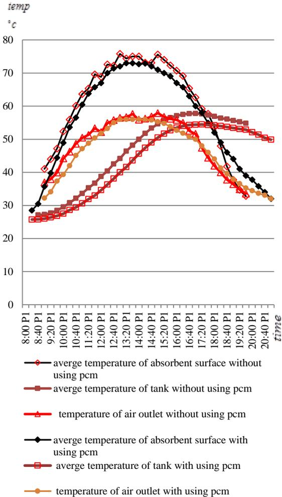
Figure 9. Comparison between the two state of with and without using PCM in thermosyphon condation. Temperatures recorded in certain hours by data logger
