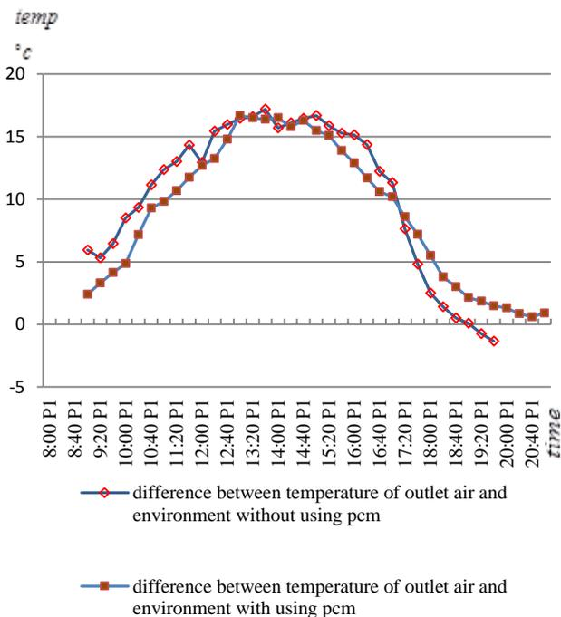
Figure 8. Comparison between temperature of air heater's outlet and environment in the two state of with and without using PCM, Temperatures recorded in certain hours by data logger
