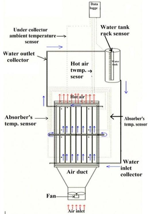
Figure 6. Schematic diagram of the experimental set-up in dual collector and thermosiphon condition
