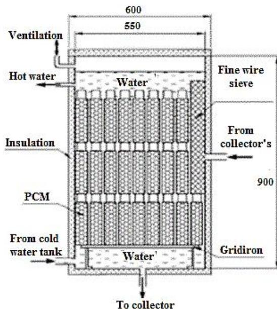
Figure 2. Cross-section of the storage unit designed [6]
