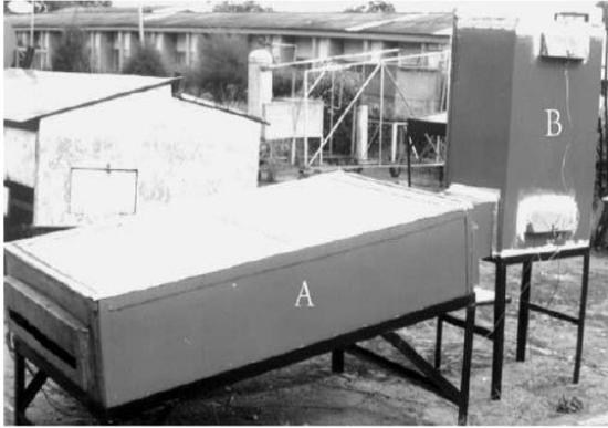
Figure 1. The air heating system: A, collector assembly with energy storage and air-heating subsystems; B, heated space [4]
