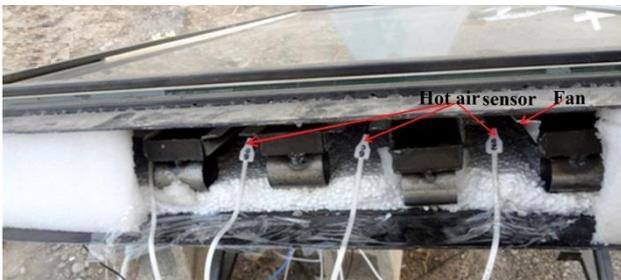
Figure 5. The hot air sensors and Feins in dual collector
