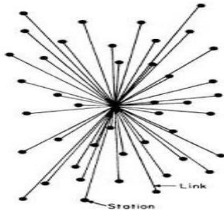
Figure 1. Centralized power networks [7]
