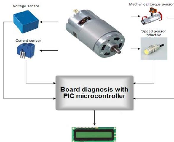
Figure 2. Block diagram of the engine diagnostic system continuous current with permanent magnets
