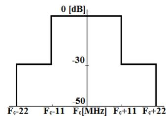
Figure 2. A diagram of IEEE 802.11 DSSS mask
