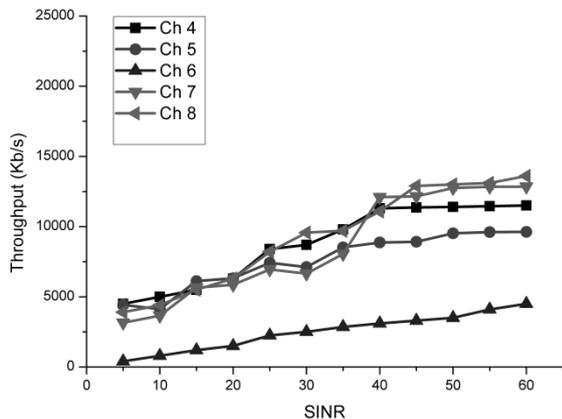
Figure 4. Throughput versus *SINR*, for 8m AP2-AP1 distance
