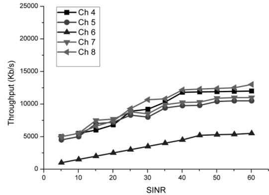
Figure 5. Throughput versus *SINR*, for 12m AP2-AP1 distance
