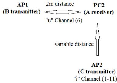
Figure 3. The equivalent scheme of the experimental platform
