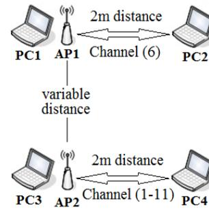
Figure 1. Experimental platform for interference evaluation
