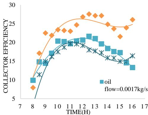
Figure 7. Instantaneous efficiency of the PTC
