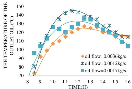
Figure 4. Changes in Outlet oil temperatures of collector during 'time'
