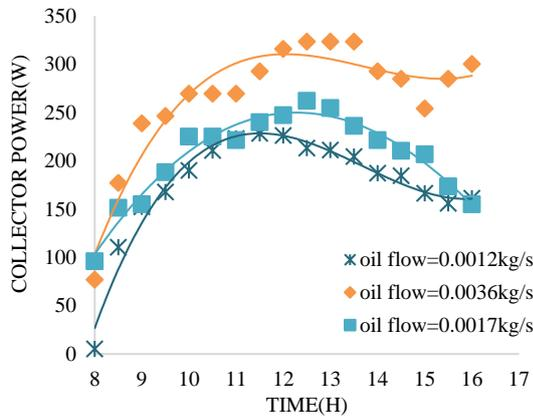
Figure 6. Power of the collector versus time
