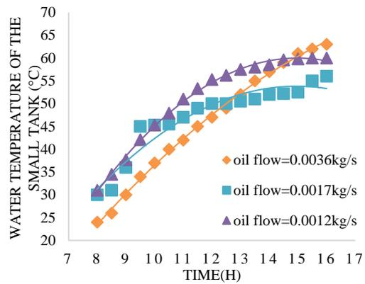
Figure 9. Temperature of small tank in terms of time
