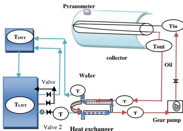
Figure 1. Schematic shape of SWHS
