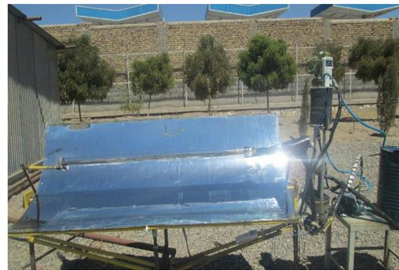
Figure 2. Image of the solar water heater system
