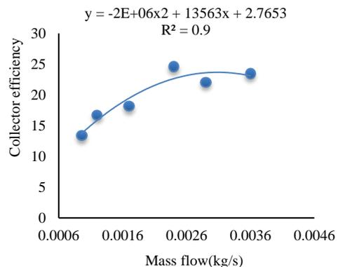
Figure 10. Variation in the collector efficiency as a function of mass flow
