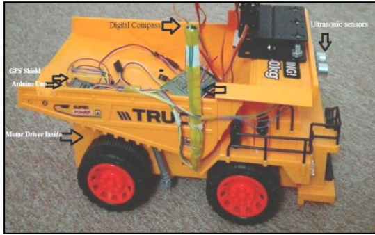
Figure 8. Toy car with GPS system
