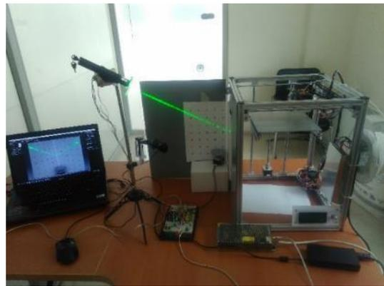
Figure 11. Implemented 3D scanner with 3D printer unit.
