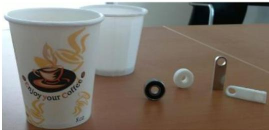
Figure 16. Original objects and their reproductions using proposed 3D-scanner/printer
