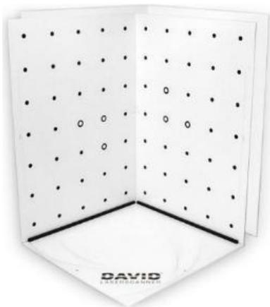
Figure 2. The calibration patterns [12]
