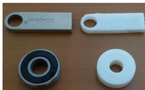
Figure 15. Original objects and their reproductions using proposed 3D-scanner/printer
