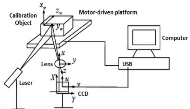
Figure 1. The block diagram of the 3D scanning with handheld Laser and Webcam - DAVID Laser scanner v3 [6]
