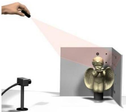
Figure 3. Scanning with a hand-held line laser [5]
