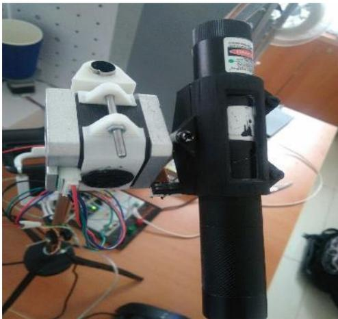
Figure 8. Laser and laser holder
