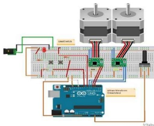
Figure 6. Circuit Diagram of microcontroller and stepper motors for scanning operation
