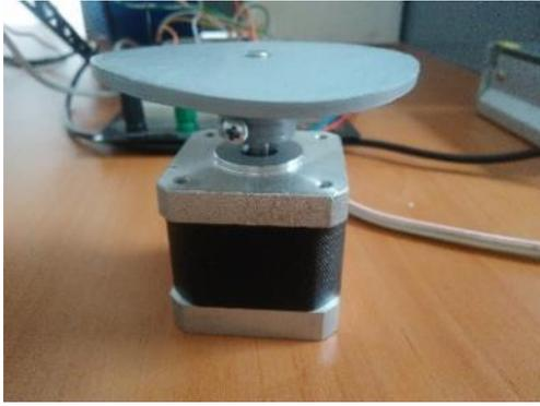
Figure 7. Platform mounted NEMA17 stepper motors
