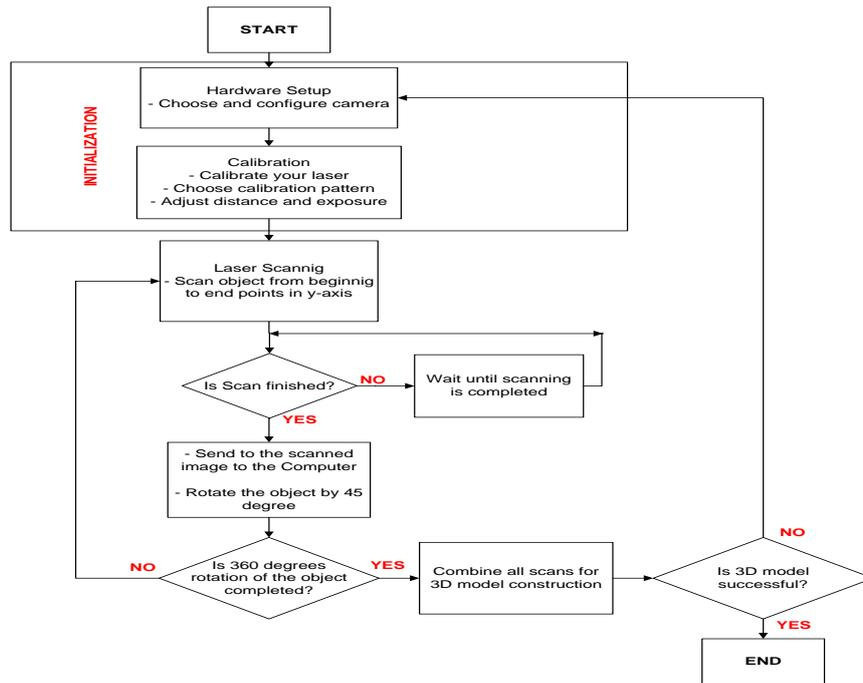
Figure 12. Flowchart for full automated scanning
