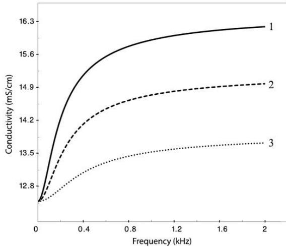
Figure 3. Dependence between the total conductivity and frequency with total capacity of double electric layer 20 µF: 1-  $R=220$  Ohm,  $R_p=70$  Ohm; 2-  $R=238$  Ohm,  $R_p=52$  Ohm; 3-  $R=260$  Ohm,  $R_p=30$  Ohm
