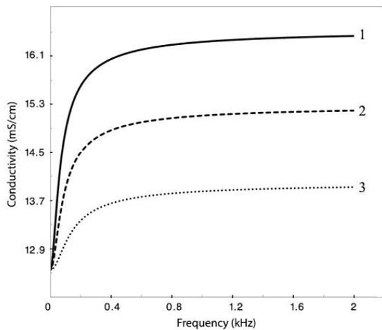
Figure 4. Dependence between the total conductivity and frequency with total capacity of double electric layer 60 µF: 1-  $R=220$  Ohm,  $R_p=70$  Ohm; 2-  $R=238$  Ohm,  $R_p=52$  Ohm; 3-  $R=260$  Ohm,  $R_p=30$  Ohm
