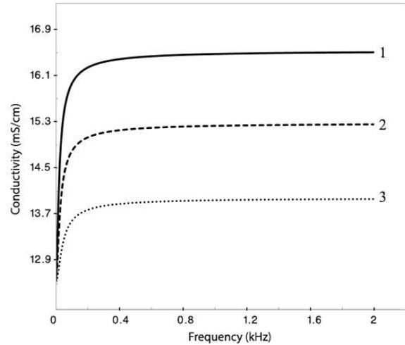
Figure 6. Dependence between the total conductivity and frequency with total capacity of double electric layer 200 µF: 1-  $R=220$  Ohm,  $R_p=70$  Ohm; 2-  $R=238$  Ohm,  $R_p=52$  Ohm; 3-  $R=260$  Ohm,  $R_p=30$  Ohm
