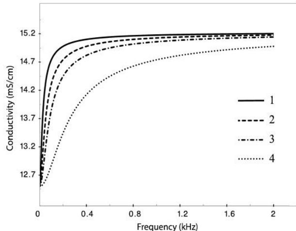
Figure 7. Dependence between the total conductivity and the frequency with active and total polarization resistance  $R=238$  Ohm and  $R_p=52$  Ohm, respectively, at the capacity of double electric layer of 1- 200 µF; 2- 100 µF; 3- 60 µF; 4- 20 µF
