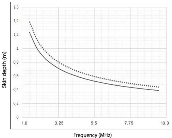
Figure 9. Dependence of the skin layer thickness from frequency  $\Delta=f(f)$
