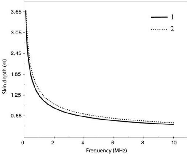
Figure 8. Dependence of the skin layer thickness from the frequency  $\Delta=f(f)$ : 1-  $\chi=0.165$  Sm/m; 2-  $\chi=0.130$  Sm/m
