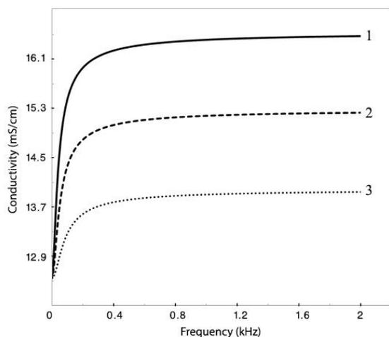
Figure 5. Dependence between the total conductivity and frequency with total capacity of double electric layer 100 µF: 1-  $R=220$  Ohm,  $R_p=70$  Ohm; 2-  $R=238$  Ohm,  $R_p=52$  Ohm; 3-  $R=260$  Ohm,  $R_p=30$  Ohm
