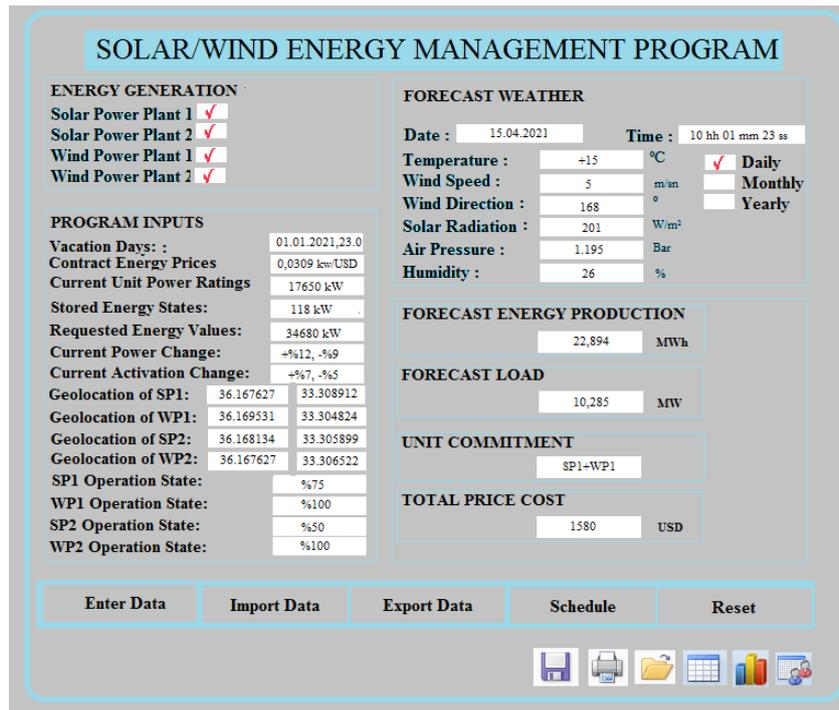
Figure 4. Solar/Wind energy management program interface
