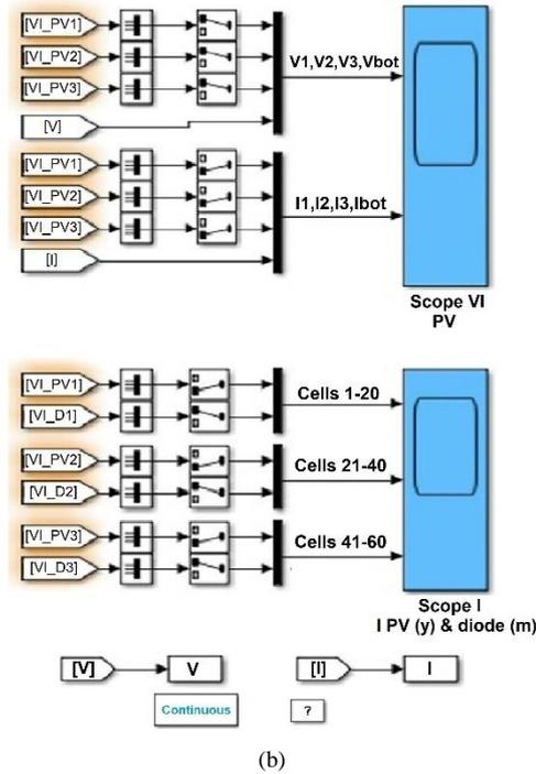
Figure 4. (a) Block diagram of a PV proposed system, (b) Partial Shading block diagram of a PV proposed system
