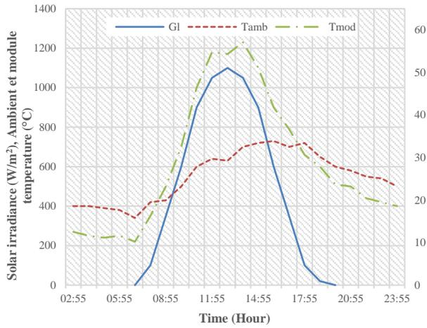
Figure 6. Ambient temperature variation, PV array temperature as well as the solar irradiance in monitoring time [10]
