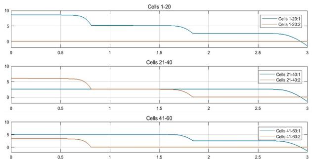
Figure 11. PV cells and diode currents characteristics
