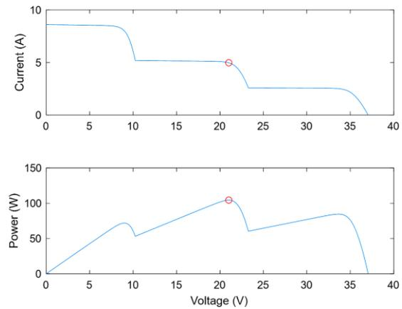
Figure 9. User defined simulation global VI and PV characteristics
