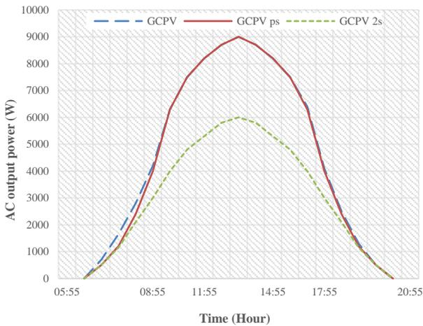
Figure 8. AC resulting power for every PV inverter for 3 PV units [10, 11]
