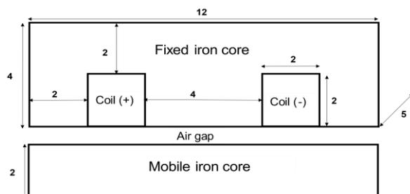
Figure 15. 2D model of electromagnet
