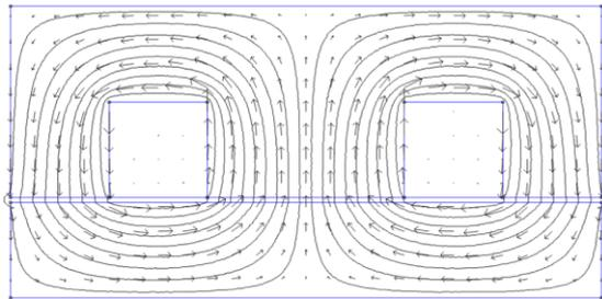
Figure 20. Equipotential lines and magnetic flux density vectors
