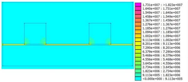
Figure 18. Magnetic field strength absolute value (legend values in A/m)
