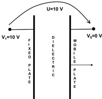
Figure 9. 2D planar model of the plate capacitor
