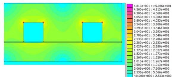
Figure 17. Magnetic flux density absolute value (legend values in T)
