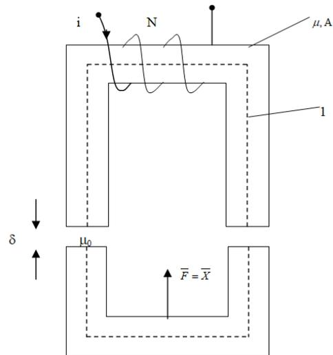
Figure 8. The electromagnet
