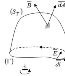
Figure 4. General domain for the electromagnetic flux law
