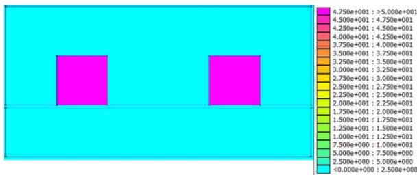
Figure 19. Current density absolute value (legend values in MA/m<sup>2</sup>)
