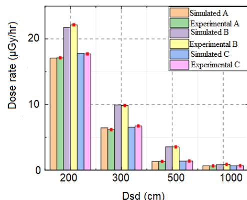
Figure 9. Dose rates simulated and experimentally at various source-detector distances [14]
