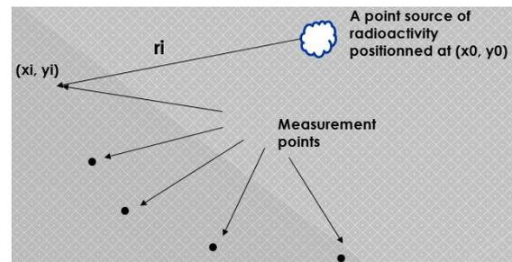
Figure 8. The geometry of the radiological point source localization issue [10]
