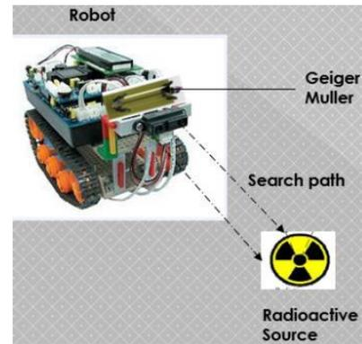
Figure 7. symbol of robot with Geiger Muller and the source
