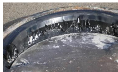
Figure 1. Wear marks on the rubber material
