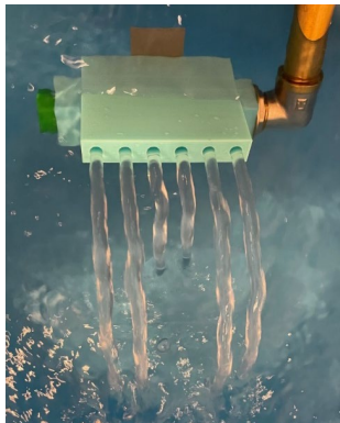
Figure 19. Demo with the diaphragm: for two ejectors in the center (No. 3 and No. 4), the diaphragm closes the inlet for the pumped medium
