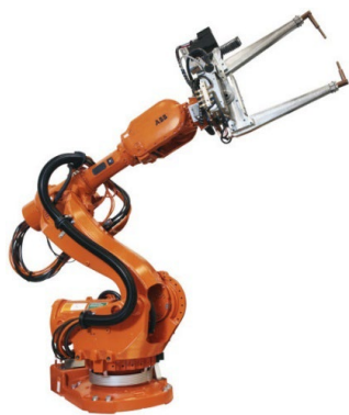
Figure 5. Robot equipped by spot-welding tong
