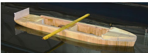
Figure 3. Model paired with a towing system
