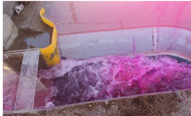
Figure 7. Flow patterns in physical model for small discharge ( H=2\text{ m} )
